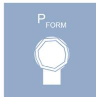
The P FORM value is the maximum permissible error for the form of a sphere. This is a value that defines the dispersion accuracy of the arm.
