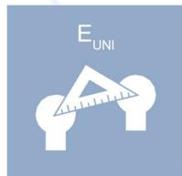
The E UNI value is the maximum permissible error for unidirectional length measurements. It therefore most closely reflects most measurement needs.
