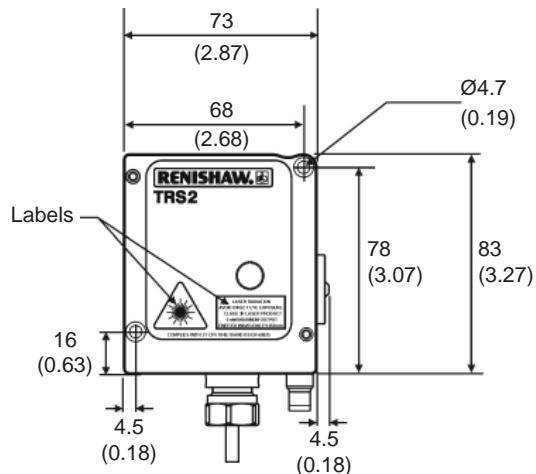
**NOTE:** These figures show a TRS2 unit. On the TRS2-S unit, the Receiver focus and Laser focus screws are not available.
